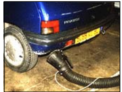
Rubber Nozzle w/nipper fixed to a car. Recommended air flow 300-600m 3 /h
