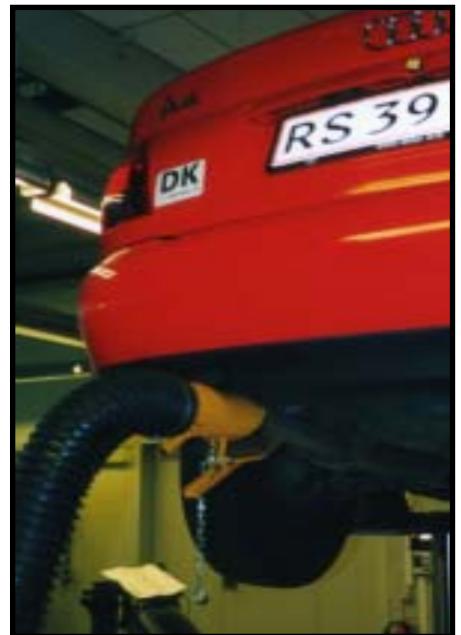
Nozzle fixed to a car. Recommended airflow volume 300 - 600 m 3
