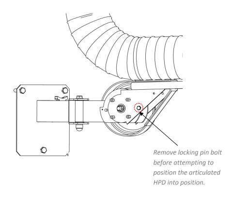
Once the locking pin has been removed the rear casing can be attached into position using the four button head bolts provided.
