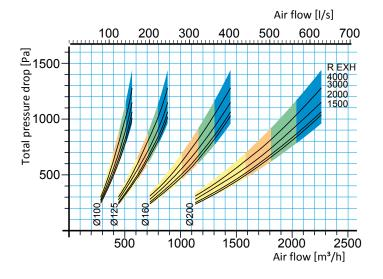
The black line shows the pressure drop for the arm when in the same position as in the design above. The area in the diagram shows the pressure drop at normal use. The field's tints show air velocity in the extractor according to below.
