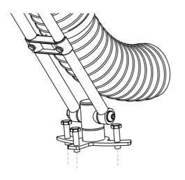
Install the bracket using 3 x M8 bolts, It is recommended that the mini arm is installed within 0.4m of the duct connection.
