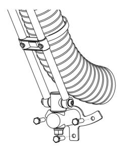
Install the bracket using 3 x M8 bolts, It is recommended that the mini arm is installed within 0.4m of the duct connection.
