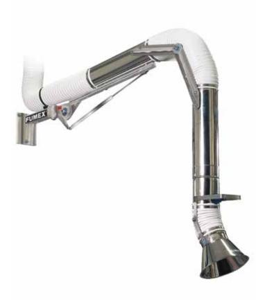
The FUMEX local extractor RX RF, with lengths 1.5, 2, 3 and 4 m, is equipped with a gas spring that balances the dead weight of the arm. For this reason, the RX RF is extremely easy to handle at the same time as it stays without rebounding when positioned, even in the outer positions. The conical hood incoporates a swivel function and may be rotated 360° and moved to a 90° angle. This allows the hood to be positioned as required.
